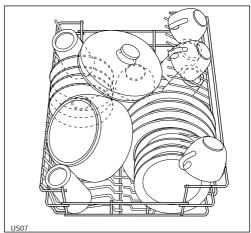
The cup-rack on the left folds upwards to increase your loading flexibility.
